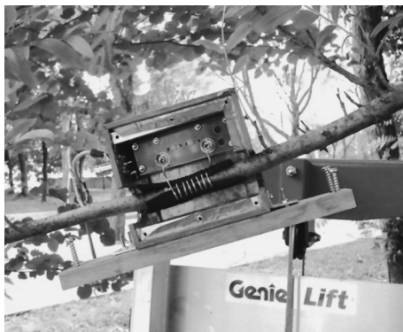
Fig. 2. RF coil and Shield BOX. RF probe was installed in the tree
