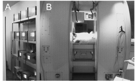
Fig. 4. (A) Light sources of fiber optic illumination in the computer room. (B) Some fibers are utilized for lighting the operation field with flexible light guides.
