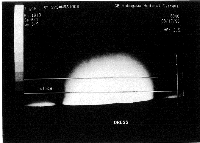
Fig. 3. Selectivity of DRESS DRESS select the volume utilizing decay of RF coil sensitivity. But total power of signal from the low sensitivity volume can not be neglected.
